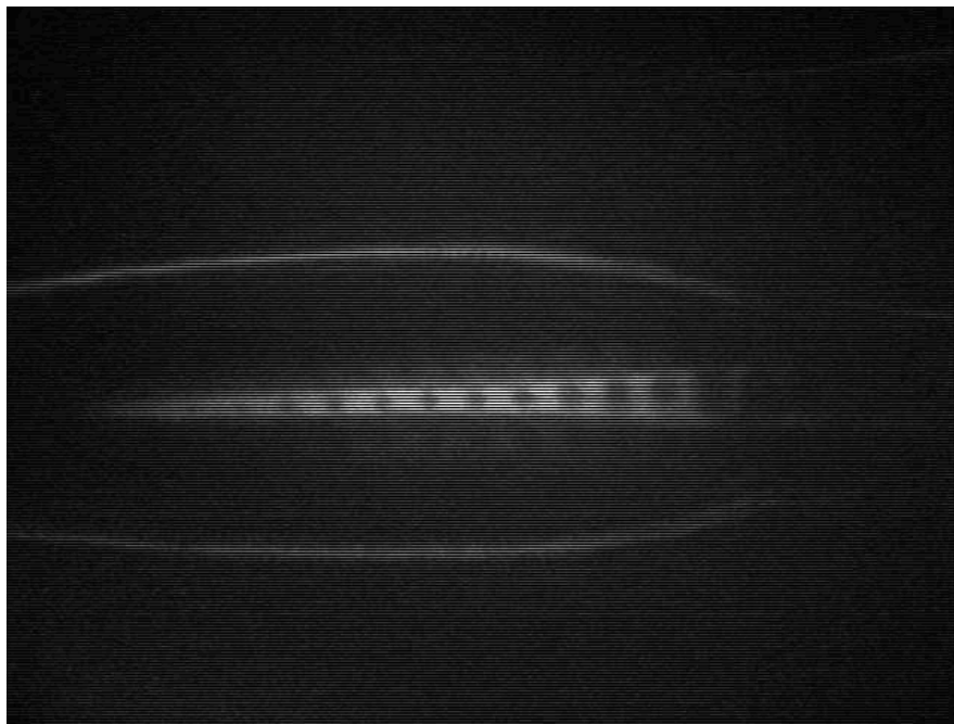
Figure I.B.8: Ar blast waves 24ns after heating beam incident with varied machining spacing. Acquired using dark field Schlieren method.
