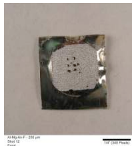
Figure I.G.2 Overview of a shot target showing the spall surface (dull area). The effect of laser intensity variations are seen from small sections of the target that did not spall.
