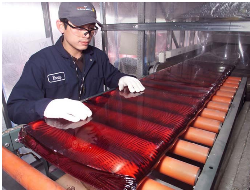
FIGURE 3.1 “Continuous melt” processed Nd-doped glass used for the National Ignition Facility. SOURCE: Courtesy of the U.S. Department of Energy.
