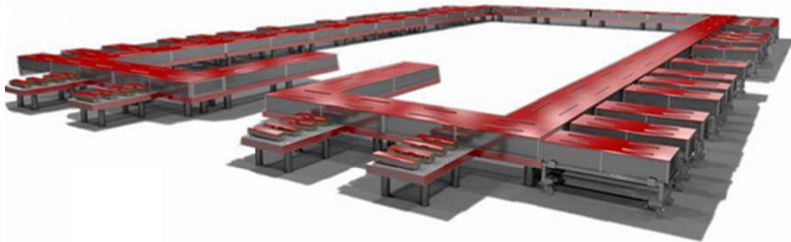
FIGURE B4.10 Computer rendition of 10-PW system to be installed at ELI-NP. SOURCE: F. Lureau, 2015, “High Power Laser System (HPLS),” in ELI-NP Science Program and Instruments Technical Design Reports , Magurele, Romania, February 18-20, http://www.elinp.ro/indico/getFile.py/access?contribId=2&resId=0&materialId=slides&confId=22 .
