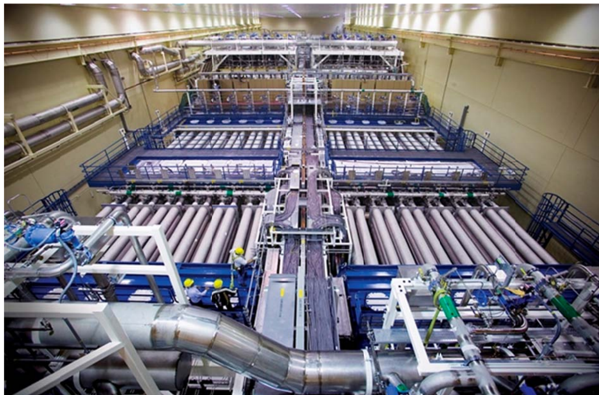
FIGURE E.5 NIF beamlines. SOURCE: NIF website laser.llnl.gov
