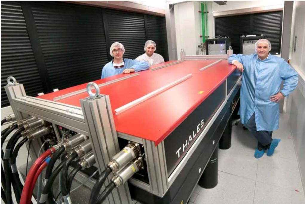
FIGURE B4.9 Photograph of ATLAS flashlamp-pumped Nd:glass laser providing 100 J of 527-nm energy at a pulse rate of 1/minute. SOURCE: F. Lureau, 2015, “High Power Laser System (HPLS),” in ELI-NP Science Program and Instruments Technical Design Reports , Magurele, Romania, February 18-20, http://www.elinp.ro/indico/getFile.py/access?contribId=2&resId=0&materialId=slides&confId=22 .
