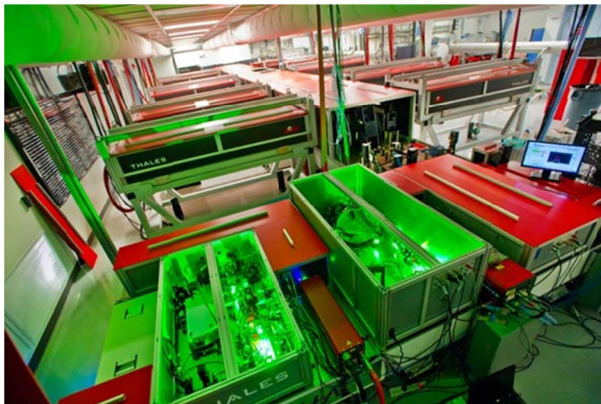
FIGURE 3.3 Nd:YAG pump laser bay of the BELLA Ti:Sapphire petawatt laser at the Lawrence Berkeley National Lab. SOURCE: http://blogs.scientificamerican.com/observations/files/2012/08/BELLA-laser.jpg .
