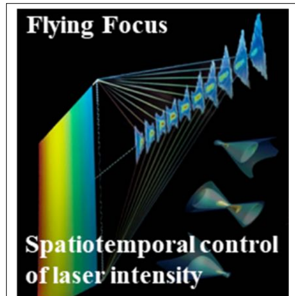
FIGURE 3.4 Focusing on the fly. A chromatic focusing system coupled to a spectrally chirped laser pulse can be used to generate a “flying focus”. This is a structure that enables a laser's peak intensity to propagate over long distances and at any velocity—including faster than the speed of light. A flying focus is produced by creating plasma lenses that focus colors at different distances with a chirped laser beam (a laser with colors that change in time). Combining such novel optical designs with plasmas is opening opportunities for laser-plasma applications including acceleration and amplification. SOURCE: Image courtesy of Dustin H. Froula, University of Rochester.
