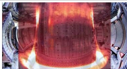
FIGURE 1.5 Record pressure in a magnetically confined plasma: In 2016, the Alcator C-Mod tokamak achieved a world record plasma pressure for magnetically confined plasmas. To achieve the record, MIT scientists employed over 4 megawatts of radio frequency heating, raising the plasma temperature to over 35 million degrees Celsius or approximately twice as hot as the center of the Sun. The C-Mod experiments reached a plasma pressure near the target value for future ITER experiments, which was enabled by new understanding of the stability properties of the boundary of the plasma. SOURCE: Courtesy of the MIT Plasma Science and Fusion Center.
