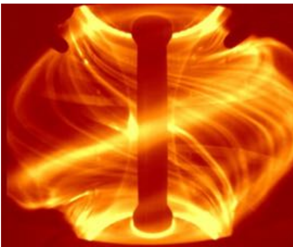
FIGURE 6.4 Edge Localized Modes or ELMs are plasma filaments that erupt from the edge of the tokamak as a result of the growth of the peeling-ballooning instability. This image shows filaments during an ELM event in the MAST spherical torus. SOURCE: © ITER Organization, http://www.iter.org/ , https://www.iter.org/newsline/229/1229
