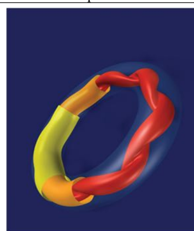
FIGURE 2.1 Seeking Minimum Energy . This image shows self-organization of a toroidal fusion plasma which spontaneously forms a helically deformed minimum-energy state. This occurs when the device is operated at high current (exceeding 1 Mega-Amperes). This particular device is a Reversed Field Pinch Experiment (RFX) at Padova, Italy. The colored nested surfaces represent magnetic surfaces reconstructed from actual laboratory measurements. The helical deformations are much stronger at the plasma core than at the edge. SOURCE: Nature Physics 5, 570, 2009).
