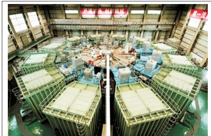
FIGURE 4.18 Pulsed Power in China. The 8 MA, 8 MJ pulsed power facility Primary Test Stand (PTS) in China is currently the largest operational pulsed power machine outside the United States. PTS has been used since 2016 to study (among other important high energy density phenomena) imploding liners (both wire arrays and solid), shock compressed materials, and behavior of a conductor under pulsed megagauss magnetic fields. PTS is about 1/3 the energy and current of Sandia’s Z machine.
