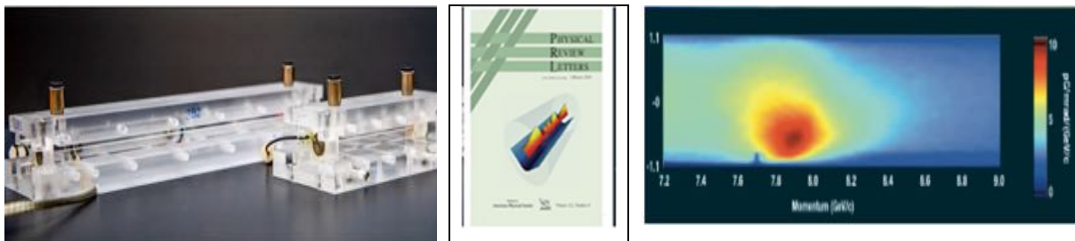
FIGURE 3.5 Laser Acceleration of Electrons to 8 GeV. (left) Compact high energy laser-plasma wakefield electron accelerators are created when an intense short pulse laser is focused plasma, here created in a capillary tube. Scaling to higher electron energies requires longer plasmas at lower plasma densities, which in turn requires new techniques for guiding the laser pulse. (center) Use of a laser to locally heat a capillary discharge plasma steepens the radial plasma density profile, enabling guiding at lower density and over longer distances. (right) This improved capability enabled production of 8 GeV electron beams at Lawrence Berkeley National Laboratory in just 20 cm of plasma, an energy conventional linear accelerators would require the better part of a kilometer to produce. SOURCE: Courtesy of Anthony Gonsalves, Lawrence Berkeley National Laboratory; middle image from Gonsalves et al., Phys Rev Letters 122, 084801 (2019).
