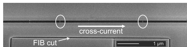
FIG. 1. SEM micrograph of the device. The trench separating the leads is the dark feature running horizontally across the micrograph and the two nanowires (circled) can be seen crossing the trench. The FIB cut and the cross-current direction are indicated.
