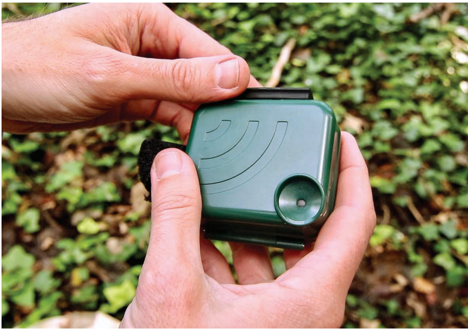
Small, ruggedized sensors, such as this passive acoustic recorder, enable remote monitoring of biodiversity. New technologies are enabling such devices to process data and transmit information via wireless networks.
