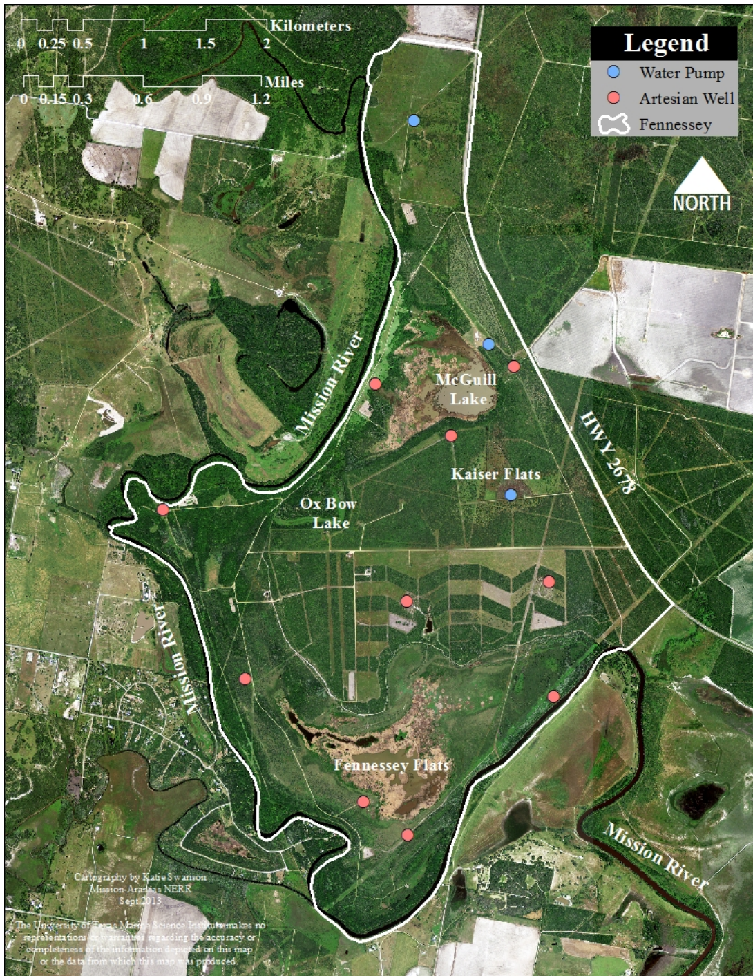
Figure 4. Location of Water Wells on Fennessey Ranch
